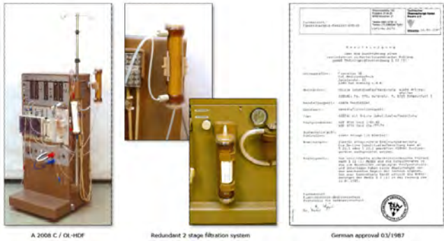
Figure 1.3. | First approved and commercially available Fresenius online HDF system for the HD machine A2008C(1987) and German approval. Source FME R&D archive.
